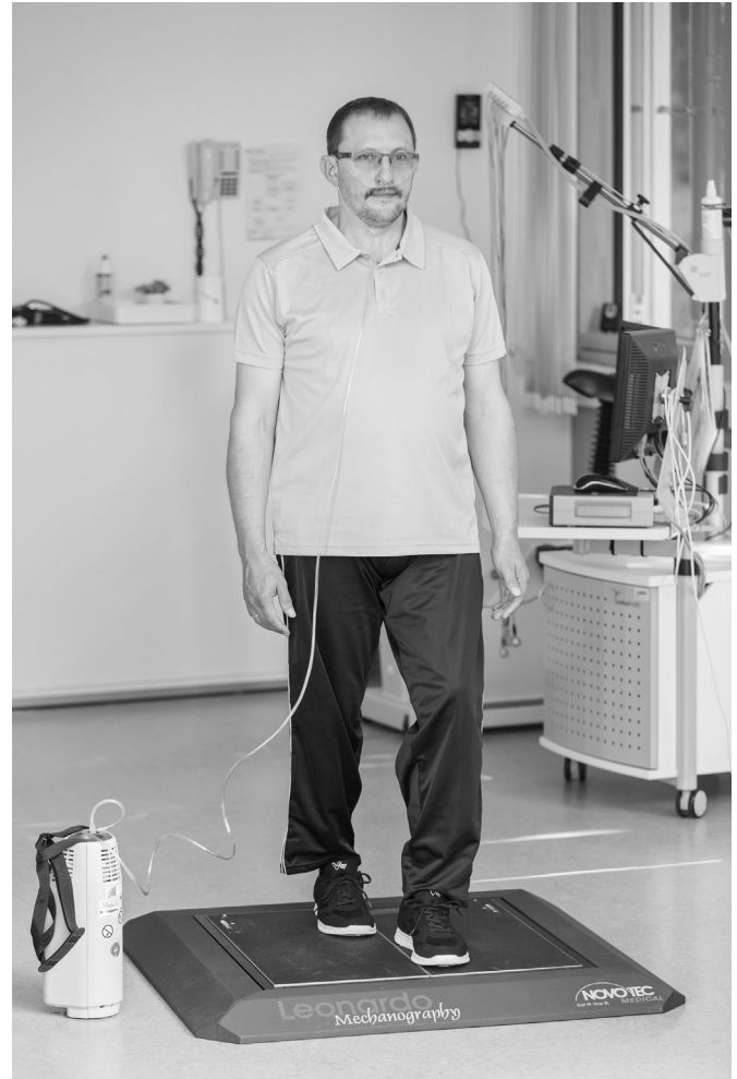
Fig. 3. COPD Patient performing a semi-tandem stance balance test on a force plate.
